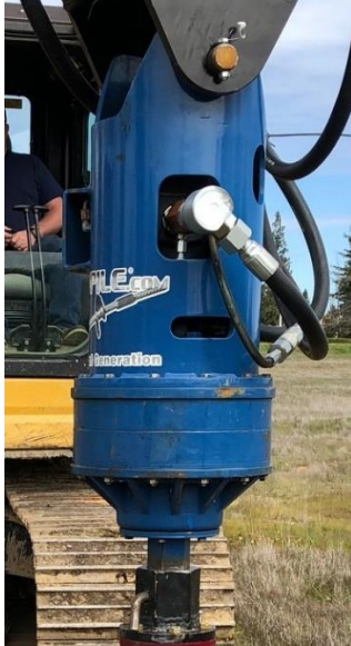
Photo 4-4 12,000 ft-lb, 420 lbs 30-60 gpm 2,850 psi max (16.3 kN-m, 191 kg) (114-227 l/m, 19.7 MPa max)
