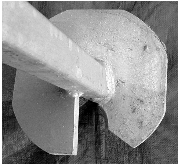
[Paper No. 2] Figure 9. Helix Leading Edge Rock Cut
