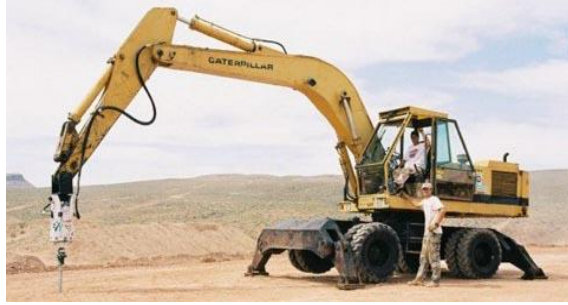
Photo 4-7 Rubber-tire hydraulic excavator capable of installing over 60 helical piles per day.
