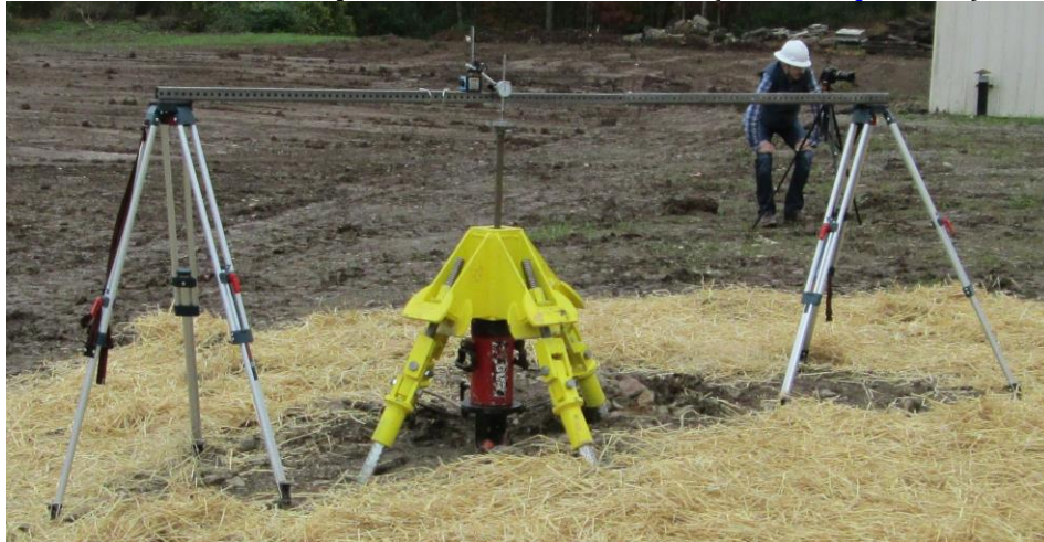
Photo 3-4 QuadPod Compression Load Test Apparatus
