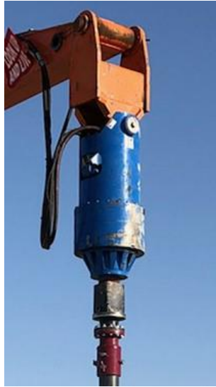
Photo 4-2 83,000 ft-lbs, 2,200 lbs, 75-185 gpm, 5,000 psi max (113 kN-m, 998 kg) (284-700 l/m, 34.5 MPa max)
