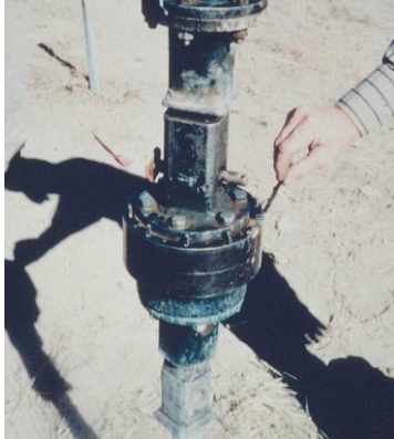
Photo 9-11 Shear-pin torque indicator (limiter).
