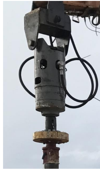
Photo 4-3 20,000 ft-lbs, 580 lbs 30-60 gpm, 2,850 psi max (27.1 kN-m, 263 kg) (114-227 l/m, 19.7 MPa max)
